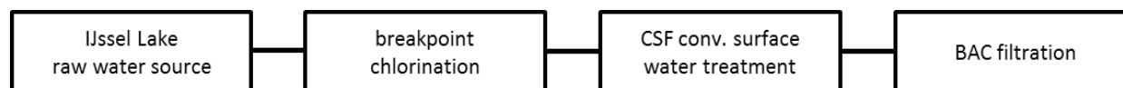
Figure 1: Treatment process scheme wtp Andijk after implementation of granular activated carbon (GAC) filtration as post-treatment in 1978
