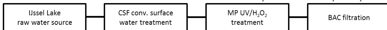
Figure 2: Process scheme wtp Andijk after implementation of MP UV/ H_2O_2 treatment in 2004
