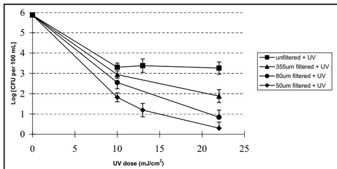
**Figure 3:** The effect of pre-filtration on survival of aerobic bacteria in UV treated water containing particles.
