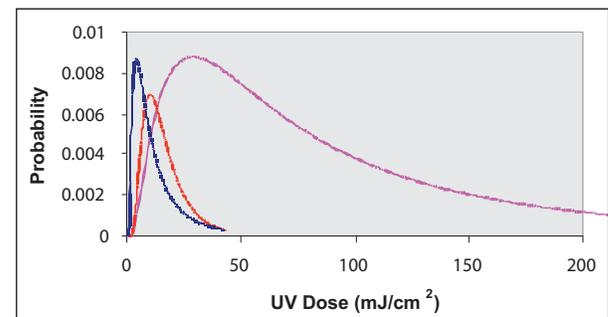
**Figure 1.** UV dose distributions determined from MS2 biosimetry.
