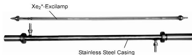
Figure 5: General view of an elevated pressure photochemistry reactor based on a DBD-driven \text{Xe}_2^* excilamp (length of excilamp: 120 cm, power consumption: 300W, UV radiation power density: 15 \text{mW cm}^{-2} , electrical efficiency: 9 – 12%)
