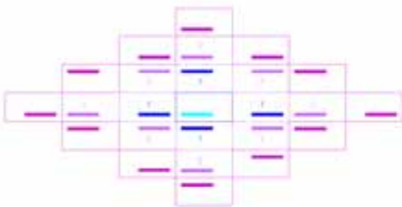
Figure 4. Schematic of the virtual image array showing the real lamp, the four first reflection images (1), the eight second reflection images (2), and a ring of third reflection images.
