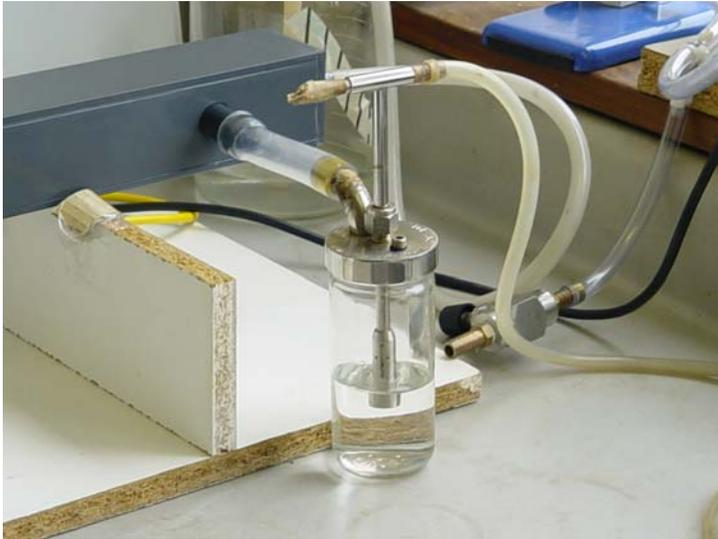
**Plate 1.** Six jet Collison nebulizer used to aerosolize the bacteria suspension
