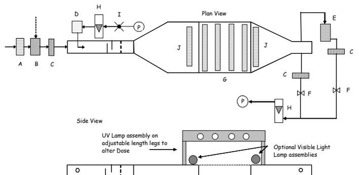
**Figure 3** Schematic diagram of the laminar flow UV exposure apparatus (A: heater, B: Humidifier, C: HEPA Filter, D: 6-jet Collison Nebuliser, E: 6-stage Andersen sampler, F: air valve, G: UV exposure section, H: tube and float flow meter, I: pressure regulator and gauge, J: visible light lamps, P: air pump).
