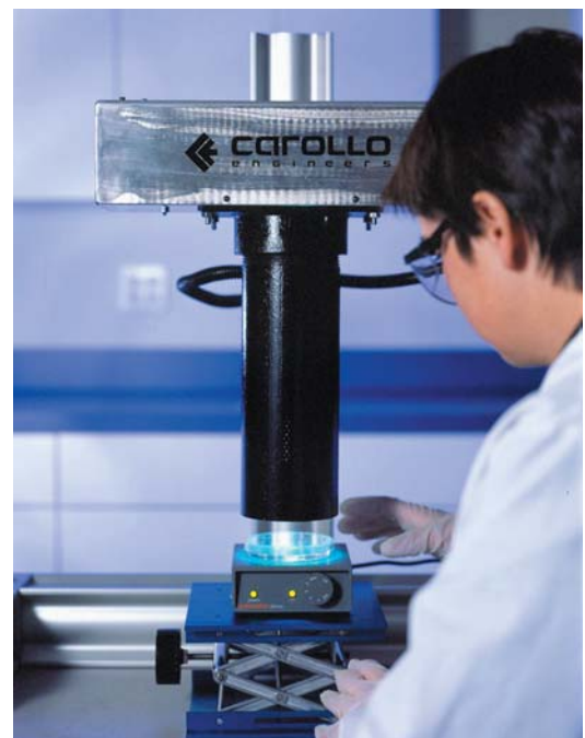
Figure 1. UV dose-response of the challenge microbe, measured using a bench-scale collimated beam apparatus, is used to relate log inactivation measured through the reactor to RED.
