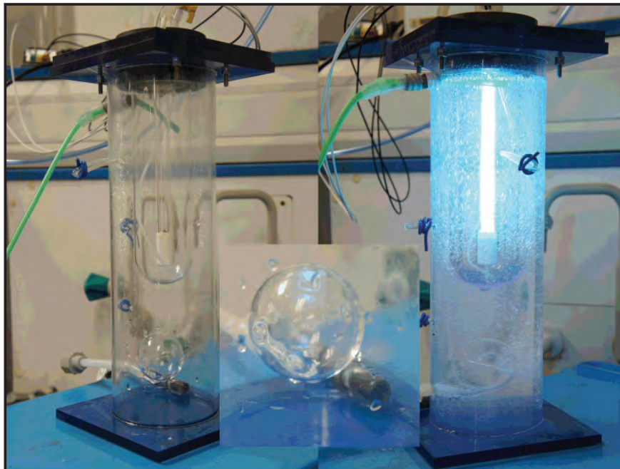
Figure 4. Photos of the reactor and the nano-bubble generator.
