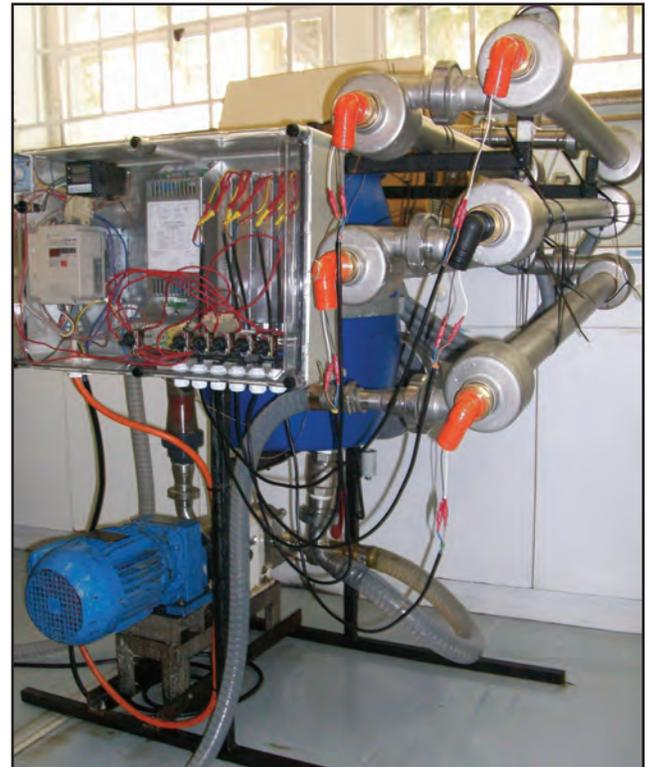
Figure 1: UV disinfection system (Sure Pure Photopurification System [SP5] lab scale model)
