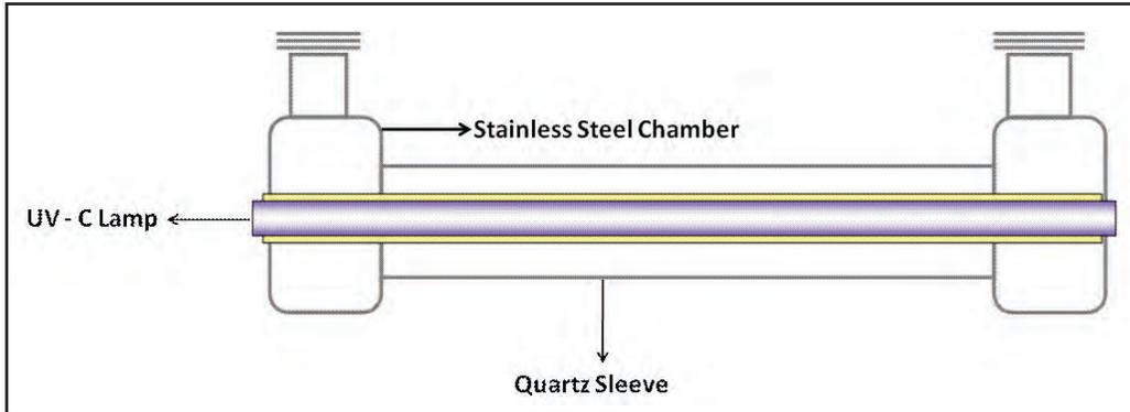
**Figure 4:** Schematic representation of the UV-C turbulator.
