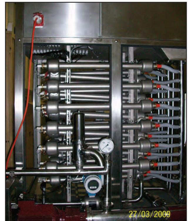
Figure 2: Sure Pure Photopurification System [SP40] commercial application
