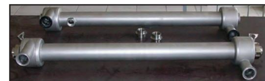
Figure 3: Single SP turbulator
