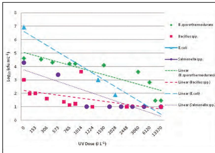
**Figure 5:** Log<sub>10</sub> reduction of various microorganisms in milk treated with UV
