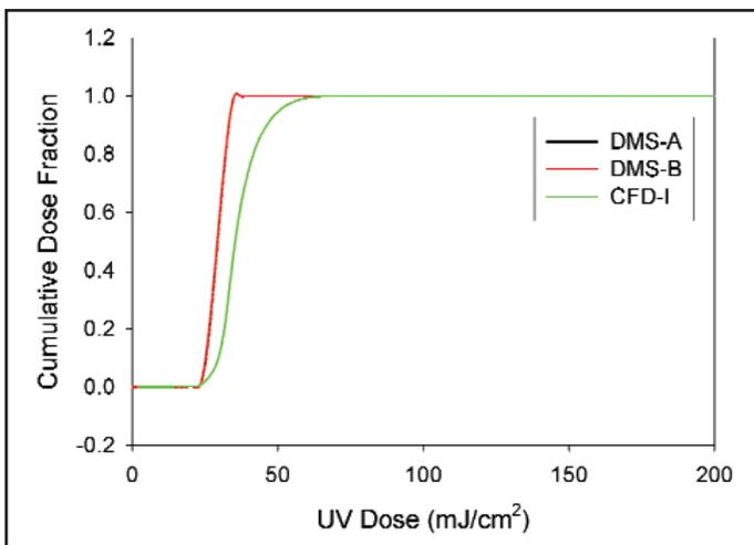
**Figure 4.** Estimates of UV dose distribution (as cumulative UV dose fraction) delivered by ITT/Wedeco reactor at operation conditions of 32 mgd (5000 m<sup>3</sup>/h), 50% power, and UVT (1 cm path length) of 90%. Note the estimates from DMS samples A and B are overlapped on top of each other.
