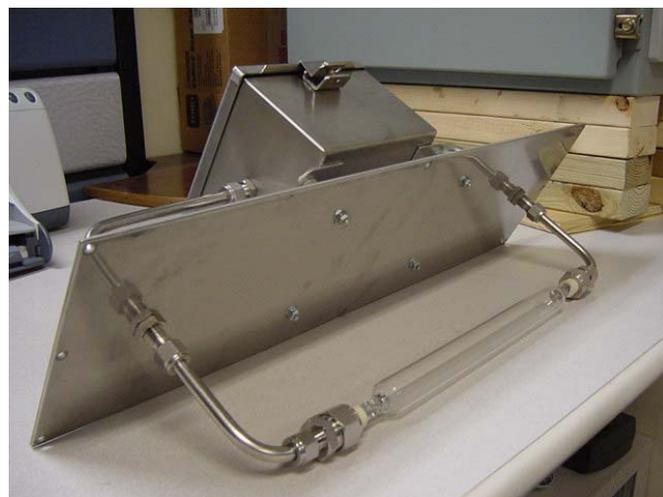
Figure 2: UV lamp installation.
